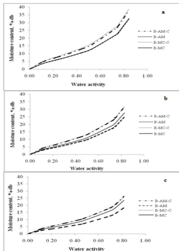
Figure 5. Effect of amylose and methylcellulose on moisture sorption isotherm of glycerol-water plasticized starch film at (a) 25°C, (b) 35°C and (c) 45°C
