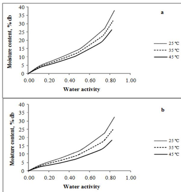
Figure 1. Effect of temperature on moisture sorption isotherm of glycerol-water plasticized starch film containing amylose (a) B-AM-C and (b) B-AM.
