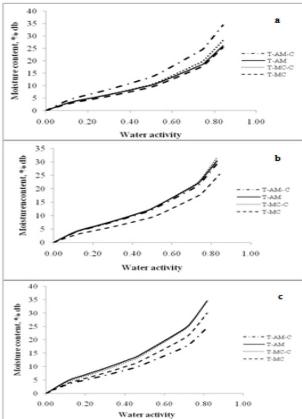
Figure 6. Effect of amylose and methylcellulose on moisture sorption isotherm of glycerol-polyethylene glycol-water plasticized starch film at (a) 25°C, (b) 35°C and (c) 45°C
