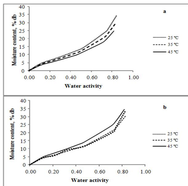
Figure 3. Effect of temperature on moisture sorption isotherm of glycerol-water plasticized starch film containing amylose (a) T-AM-C and (b) T-AM.
