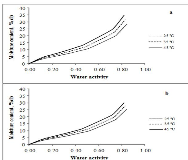
Figure 4. Effect of temperature on moisture sorption isotherm of glycerol-water plasticized starch film containing methylcellulose (a) T-MC-C and (b) T-MC
