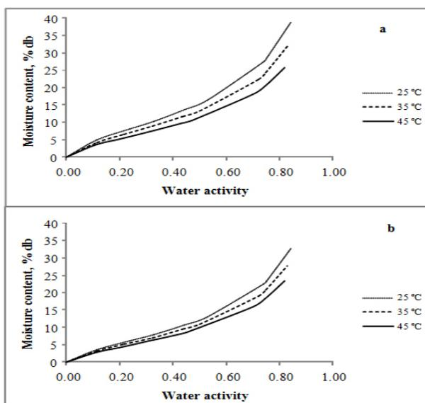
Figure 2. Effect of temperature on moisture sorption isotherm of glycerol-water plasticized starch film containing methylcellulose (a) B-MC-C and (b) B-MC
